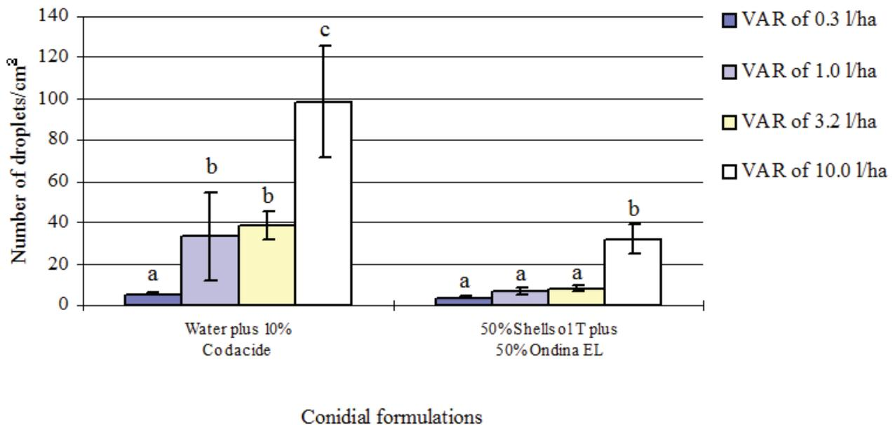
Figure 3. Number of droplets/cm<sup>2</sup> ( $\pm$  s.e.) of two conidial formulations sprayed at different equivalent VARs with a spinning disc atomiser working at 6030 rpm and counted on water and oil-sensitive papers. Note: Means followed by the same letter within the same formulation are not significantly different ( $p < 0.05$ ).
